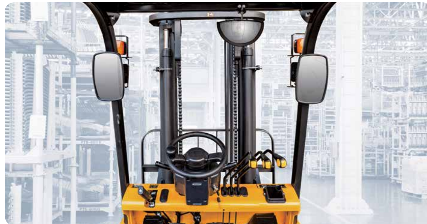
Wide view mast
