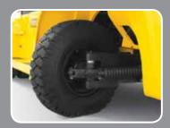
Fully hydrostatic power steering
