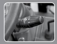
**Multi-function switch lever** Multi-functional switch lever gives
